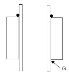
The optimum volume of brazing alloy required in a joint is 25% more than the volume of the joint gap at the brazing temperature.
